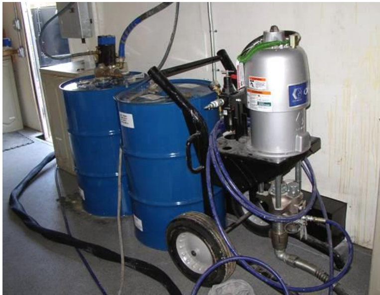
Figure 1: Suction tube feed from material drum (photo courtesy of Gaco)
