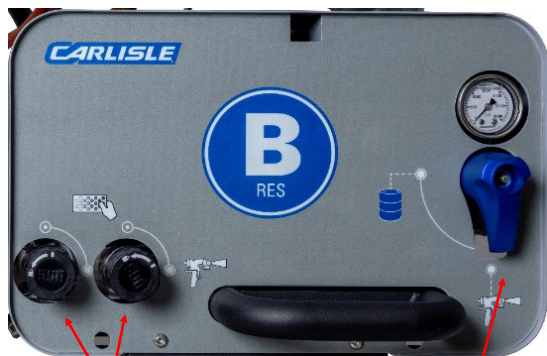
Filter inlet and outlet valves in open position
